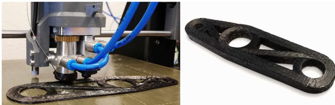
Figure 4.50: 3D Printing with Endless Fiber Reinforcement and Final Part (Courtesy of 9T Labs)
