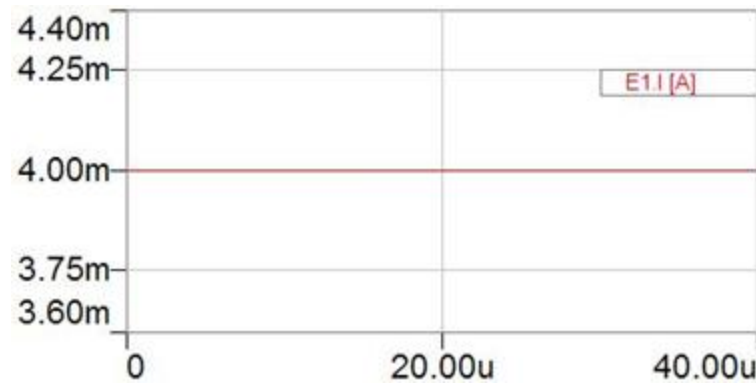
Figure 4. Simulation results-supply current of ABS_PRESS_PE1
