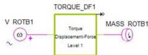
Figure 2. Application example of the Torque Sensing (Displacement-Force) block
