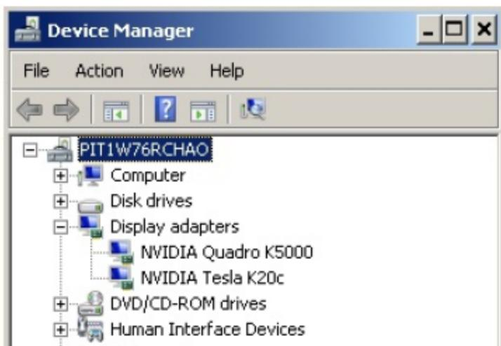
2. You should run nvidia-smi.exe at C:\Program Files\NVIDIA Corporation\NVSMI or C:\Windows\System32 to check if GPU cards are installed successfully. The executable nvidia-smi.exe should exist after the display driver is installed.
