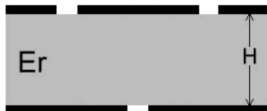
Substrate Layer With Overlay Capacitors and Interlaced Resonators
