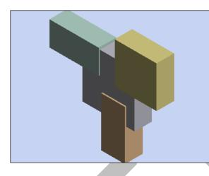
For this setting, the application displays the model as bounding boxes that are aligned by the X, Y, and Z axes of the coordinate system. This changes the appearance of complex structures that are not well-aligned with the axes. This setting significantly improves model drawing and rotation speeds, especially for complex models.
